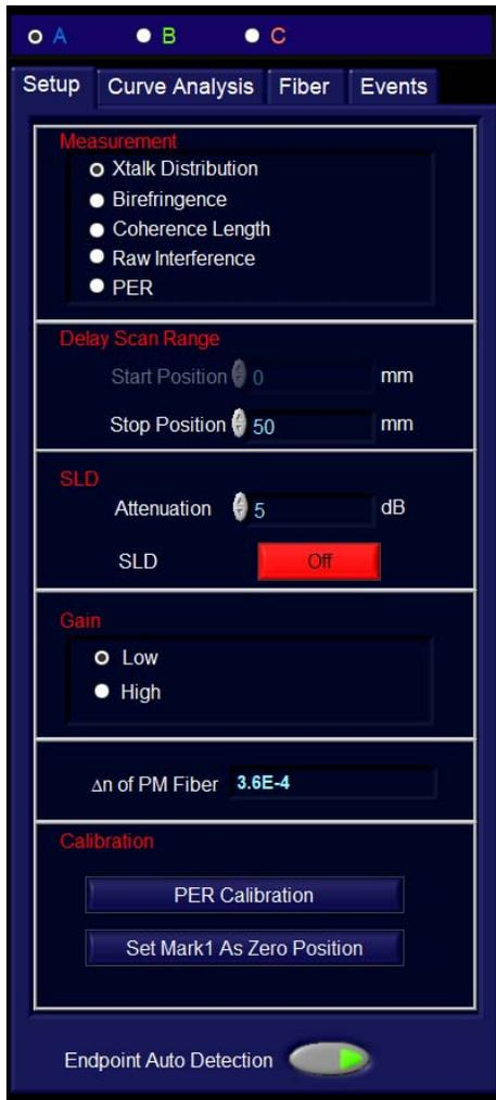
3. Select "Xtalk Distribution" from the Measurement menu on the Setup tab.
