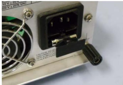
**Figure 5 Fuse compartment**
