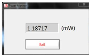
Check that the optical power is at an appropriate level. Power  $\sim 1\text{mW}$  or so usually works well. If the power is too high or too low, change the power level of the light source (if possible) and check the power again.
