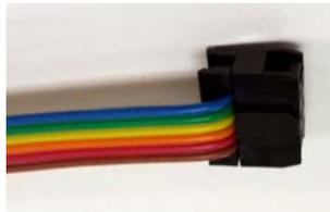
**Figure 12 PSW driver board electrical cable**
