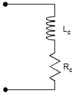
**Figure 4 PSW-002 equivalent electrical circuit**
