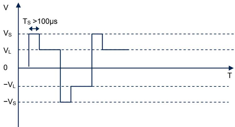
**Figure 5 Drive signal diagram**
