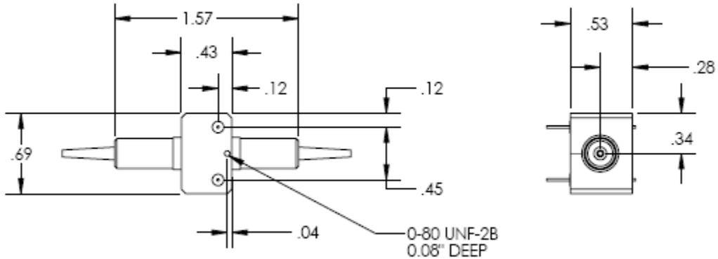
**Figure 8 Dimensions and mounting hole information**
