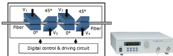
Fig. 2 Illustration of a multifunction polarization controller (MPC-202) constructed with multiple fiber squeezers.
