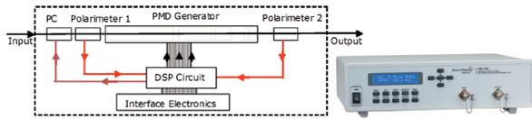
Fig. 5 Illustration of PMDPro™ polarization optimized PMD source. Its PMD generator can generate 1<sup>st</sup> and 2<sup>nd</sup> order PMD in less than 1 ms. The polarization controller (PC) is used to generate different SOP variations as in the MPC-202. In addition, the PC, together with the two polarimeters, is used to perform polarization optimization functions as well as polarization synthesis functions.
