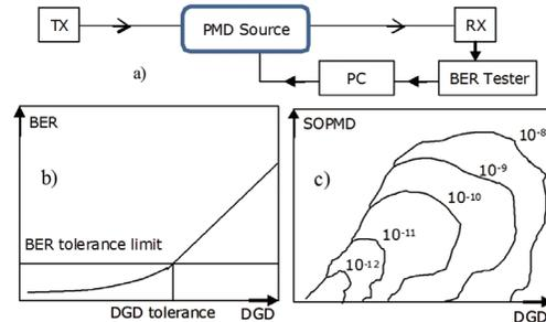
Fig. 7 a) PMD tolerance test setup using a PMDPro™ PMD source. The computer (PC) selects PMD settings and collects BER readings. b) A BER vs. DGD curve can be obtained, and the DGD tolerance for a given BER threshold can be deduced using the curve. c) Map of BER vs. DGD and SOPMD. Each contour represents a BER value, and the PMD tolerance can be obtained from the contour plot.
