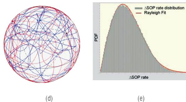
Fig. 3d) SOP trace generated by the Rayleigh scrambling function.
