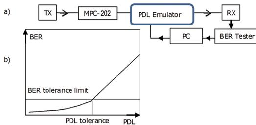
Fig. 8 a) PDL tolerance test setup. b) A typical BER vs. PDL curve
