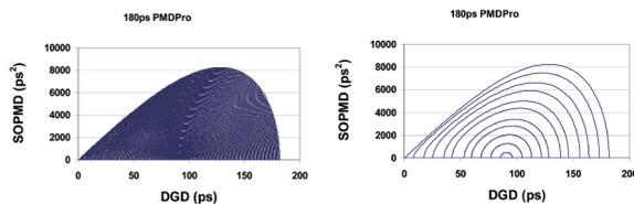
Fig. 6 The left plot is a comprehensive map of DGD vs. 2<sup>nd</sup> order PMD (SOPMD), showing the coverage of generated PMD values with dense (256) PMD traces. The right plot shows some typical PMD traces. PMD values can be varied quickly along those traces.
