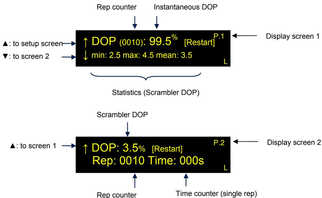
On display screen 1, the top line contains the rep counter, which counts up scrambler DOP measurements as they are completed, and an instantaneous DOP measurement display. The instantaneous DOP is the measured DOP corresponding to the polarimeter's basic SOP measurement, not the time-averaged scrambler DOP. The bottom line shows the running statistics (min, max, and mean) for scrambler DOP measurements. These will be updated until all measurements are completed.
