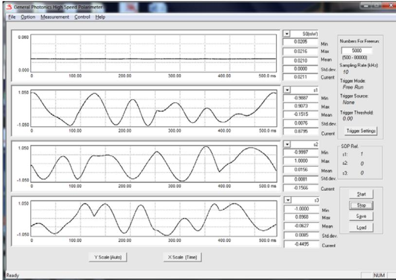
This option displays data on a virtual oscilloscope window and allows for triggered measurement.
