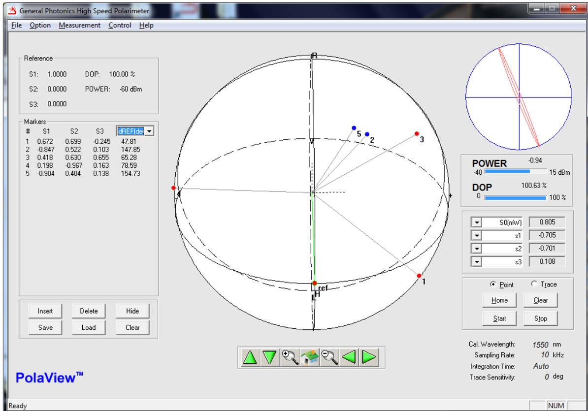
This option allows the user to mark points on the sphere and measure the angles between marked points or between marked points and a reference SOP. Up to 99 points can be marked. Selecting the Marker option from the Measurement menu causes the Marker control pane to appear on the left side of the screen.
