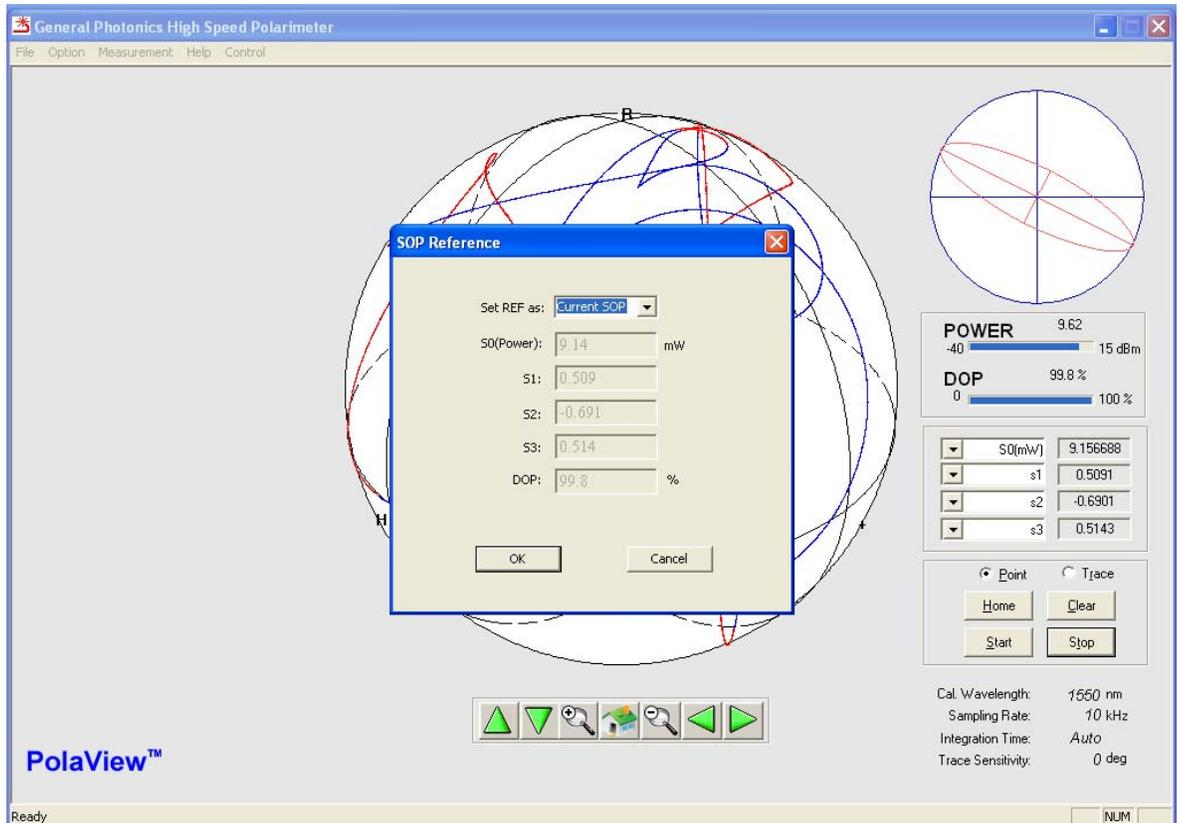
For "current REF", the reference Stokes parameters, power level, and DOP stored in the instrument are used. This is the default setting.
