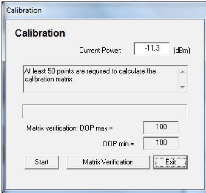
Click "Start" to begin matrix generation. Move the fiber or use a slow polarization scrambler to create the required set of diverse SOPs.
