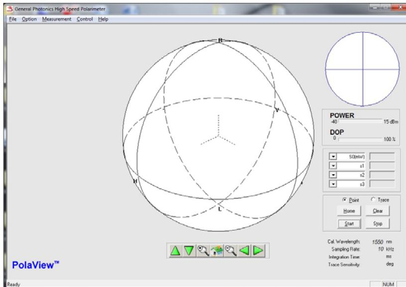
This option displays data on a Poincaré Sphere. It is the default data display mode.
