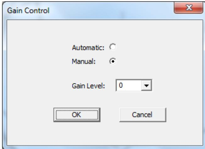
The gain control window allows the user to set the gain control mode to automatic (gain level may vary with power level) or to manually set a fixed gain level (0 to 18).
