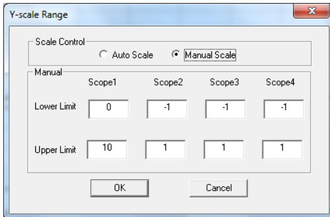
In Oscilloscope mode, PolaView has 4 scope windows. The Y-Scale Range setup allows the user to configure the Y axis for the scope traces.
