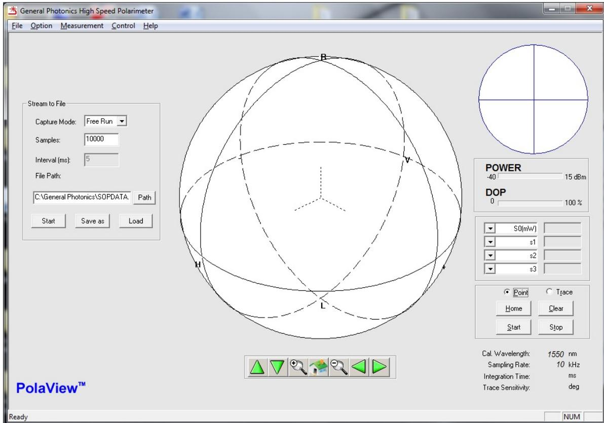
The “stream to file” function saves measured data to one or more text files, as well as displaying it on the sphere. Selecting this option from the Measurement menu causes the “stream to file” control pane to appear on the left side of the screen.
