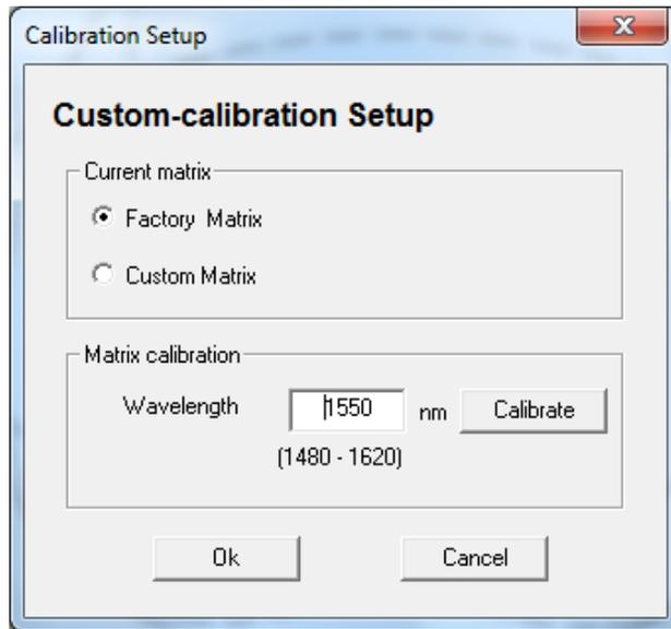
The calibration setup window allows the user to select the polarimeter calibration matrix to be used for SOP measurement.
