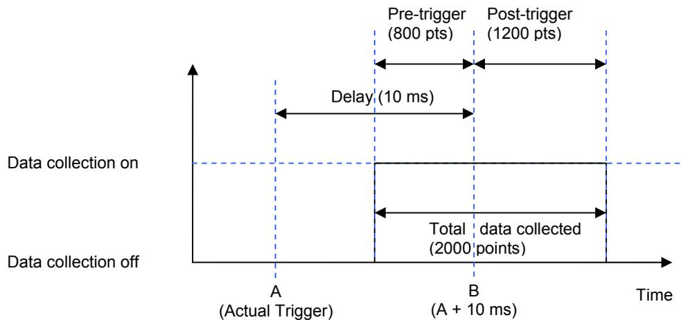
**Figure 19 Triggered measurement timing diagram with example values.**
