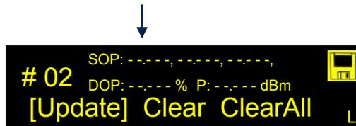
The user can also clear or update existing data. The ◀▶ buttons move the cursor between the "Update", "Clear", or "Clear All" options and location selection. From the "Update" option, the ◀ button moves the cursor to the storage ID number. The ▲▼ buttons change the value of the selected digit. If there is data stored at a particular location, it will be displayed in the data fields.
