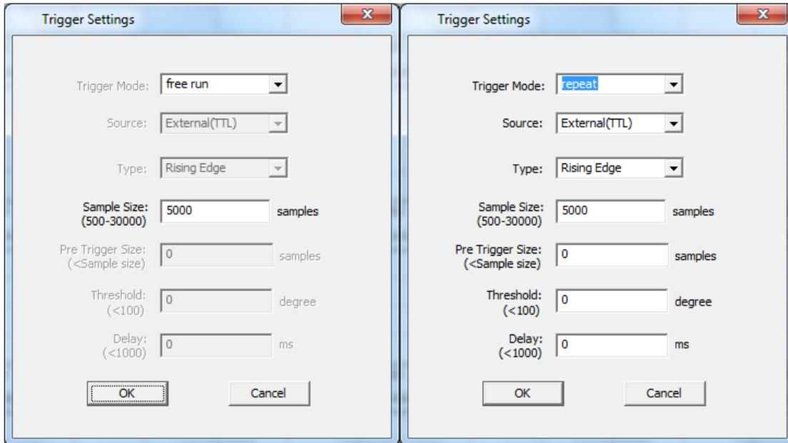
The Trigger Settings window allows the user to set up parameters for triggered measurement in oscilloscope mode.
