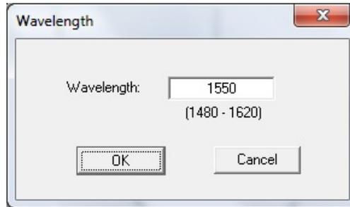
The wavelength setting determines the calibration matrix used for SOP measurement.
