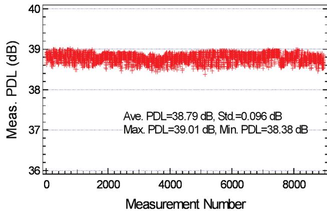
Figure 2. Measurement of high PDL sample: Polarizer
