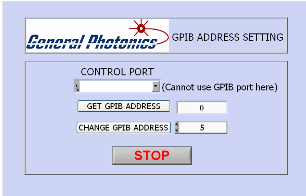
Figure 11 Retrieve or change the GPIB address via LabView program
