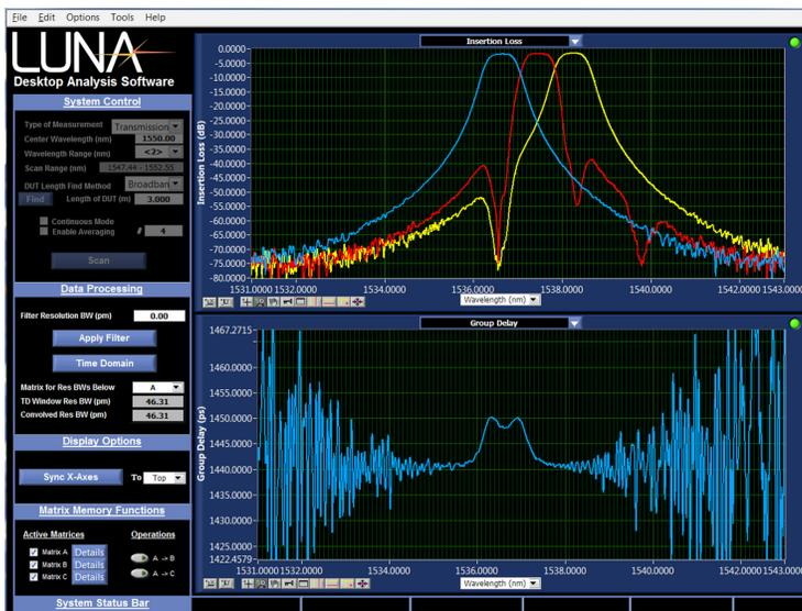
With a single scan, the OVA 5100 simultaneously measures the complete transfer function of photonic components. This screen shows IL and Group Delay versus wavelength.
