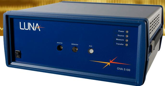
The Luna OVA 5100 is the fastest, most accurate and economical tool for loss, dispersion and polarization analysis of modern optical devices and systems, including photonic integrated circuits (PICs).
