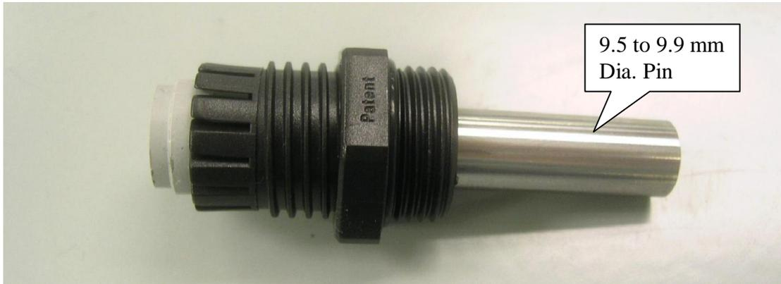
**Figure 4 . Removing Seal with Pin**
