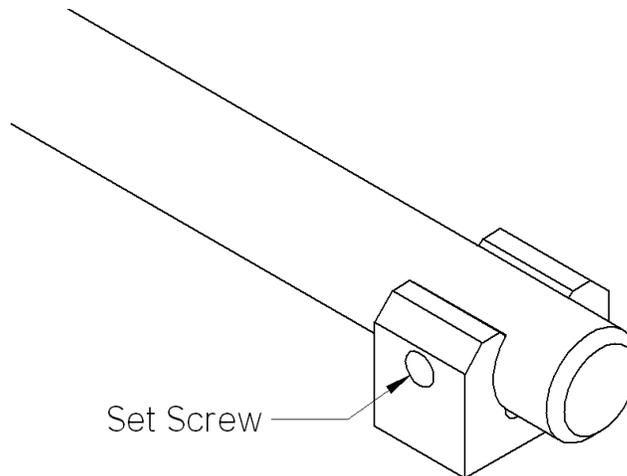
Figure 3 – Close up of mounting bracket & Setting Bar
