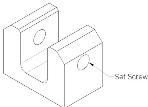
**Figure 1 – Mounting Bracket**
