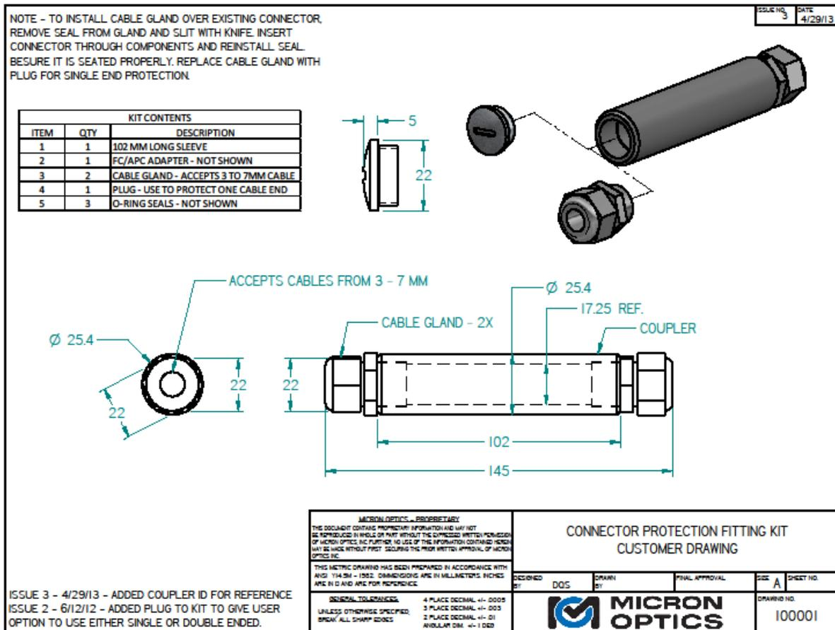
**Figure 18 – Universal Connector Protection Fitting**
