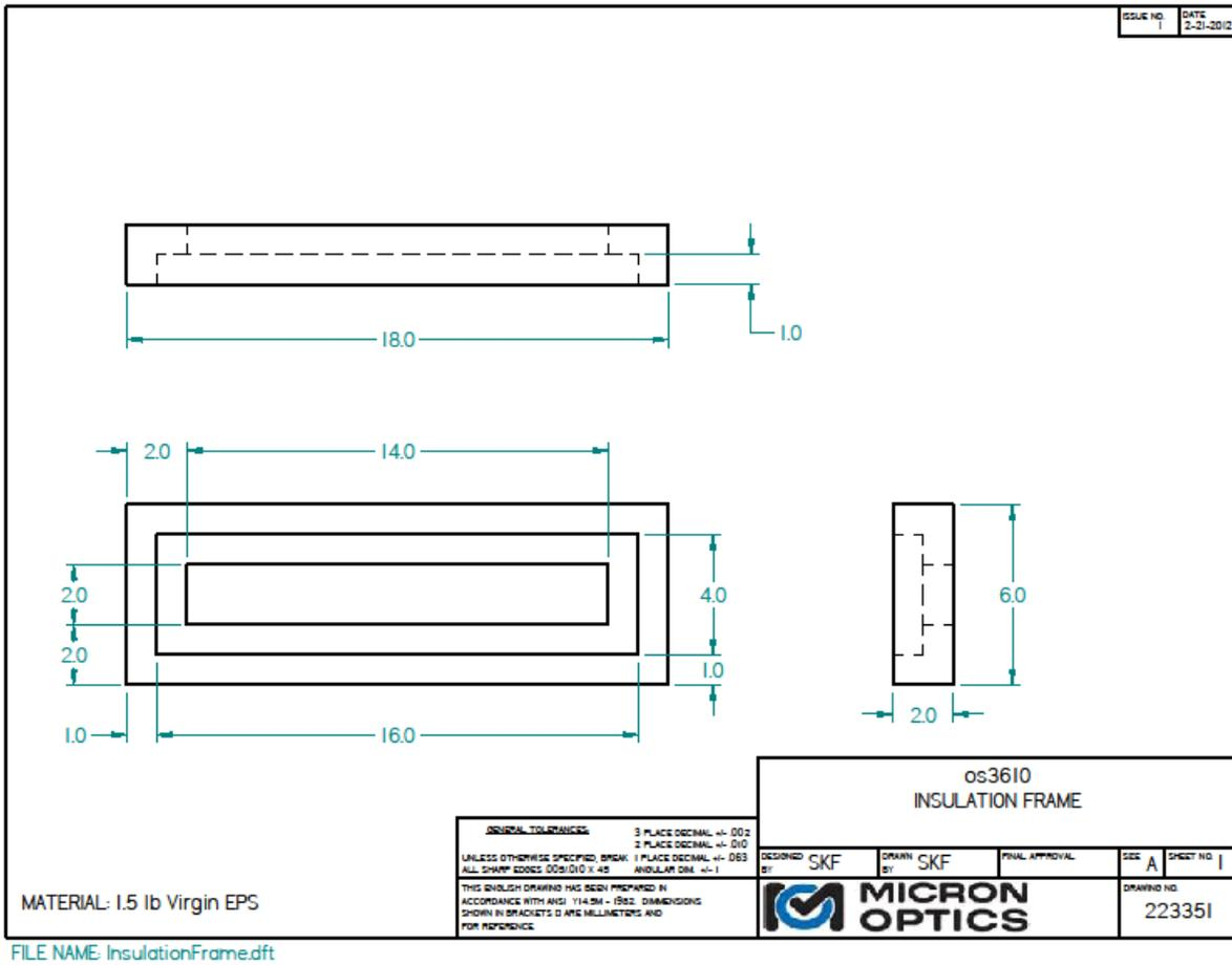
**Figure 16 – Insulation Frame**
