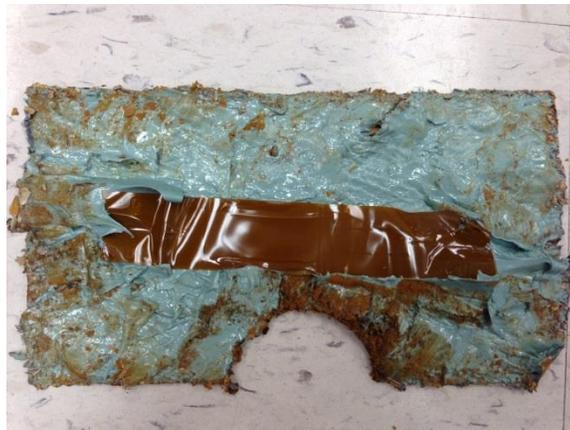
**Figure 6 – Removed STOPAQ**
