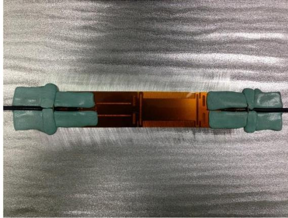
**Figure 9** – STOPAQ Paste Detail
