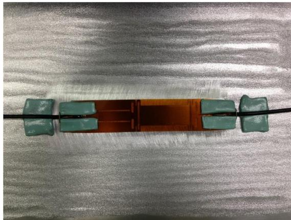
**Figure 8 – STOPAQ Paste on End of Gage**
