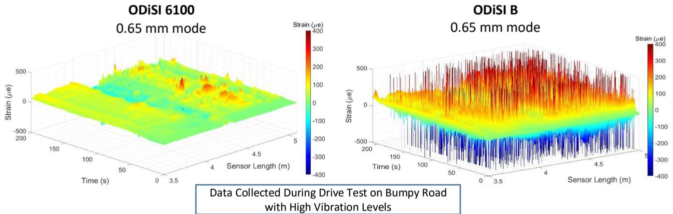
The high value data outliers in the ODiSI B data (red and blue spikes) represent invalid data due to the high levels of vibration and movement present in the sensor. The impact on the ODiSI 6 measurements were much lower.
