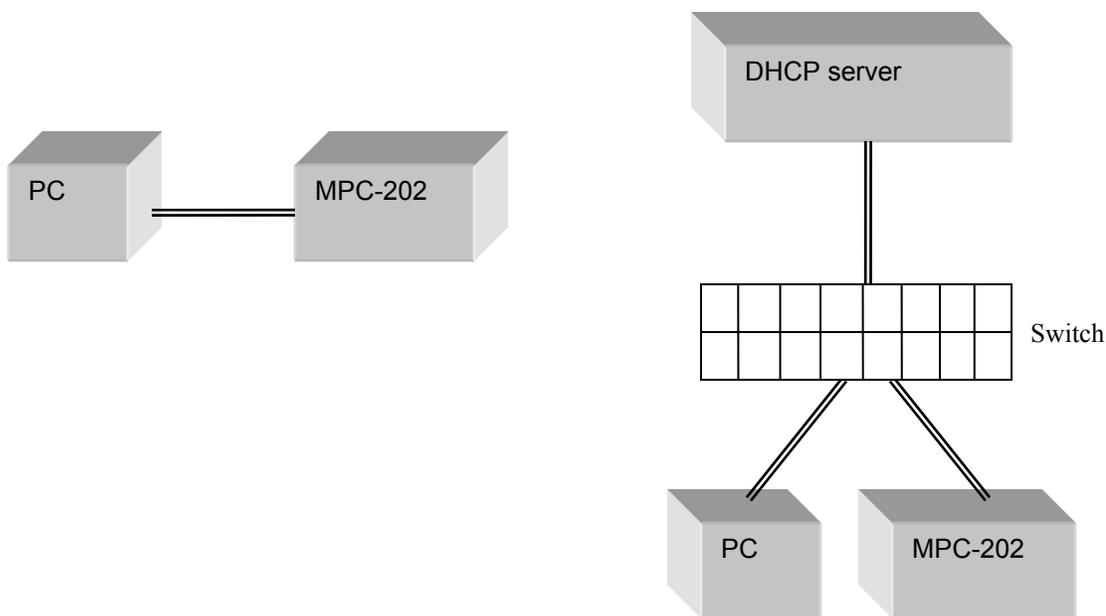
**Figure 28 Direct connection: MPC-202 to PC**
