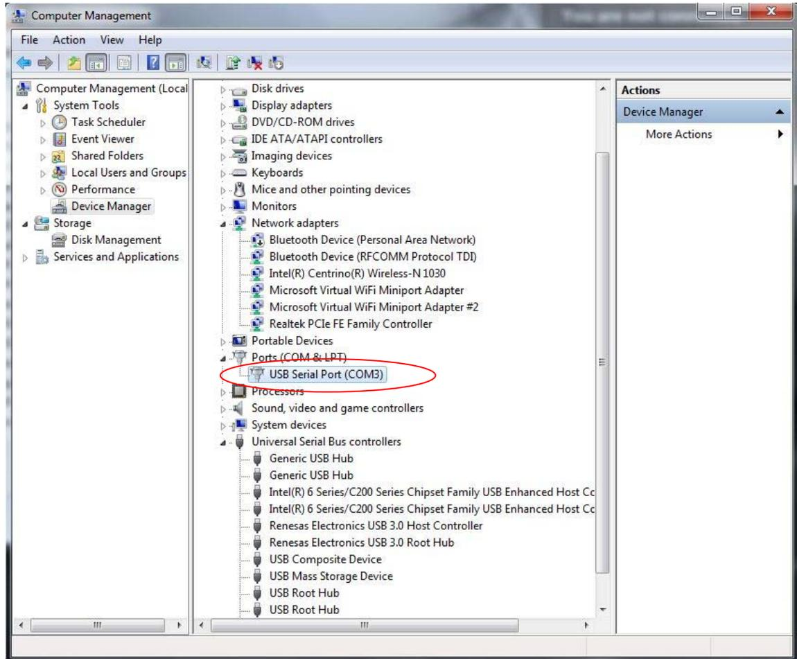
Note the port number that the MPC-202 is using (COM3, in this example).
