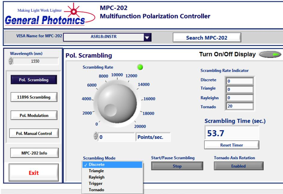
Scrambling mode selection: Select the desired scrambling mode from the pull-down menu at the bottom center of the screen:
