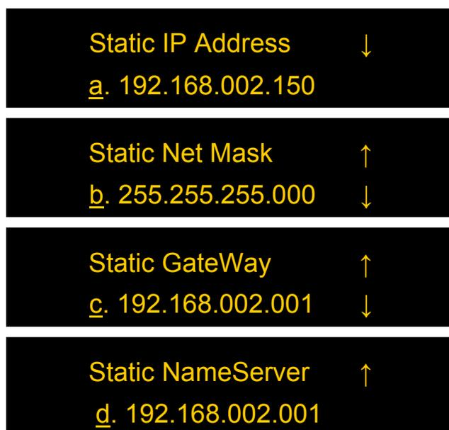
Rotate the wheel to move between static IP setup parameter options when the cursor is on the setup parameter index (a-d).
