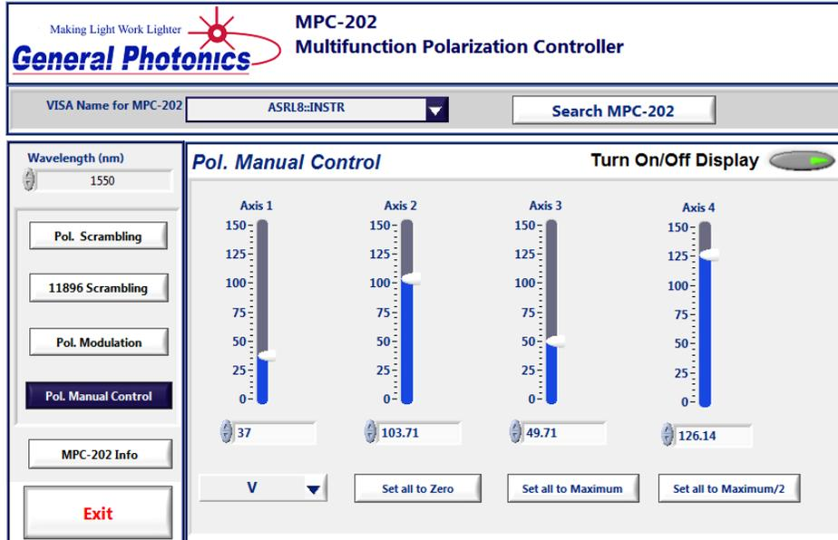
Individual channel controls: Tune the control voltage of each channel by dragging the slider, using the arrow buttons, or typing a value in the box and then pressing ENTER on the keyboard. Range is determined by the selected units.
