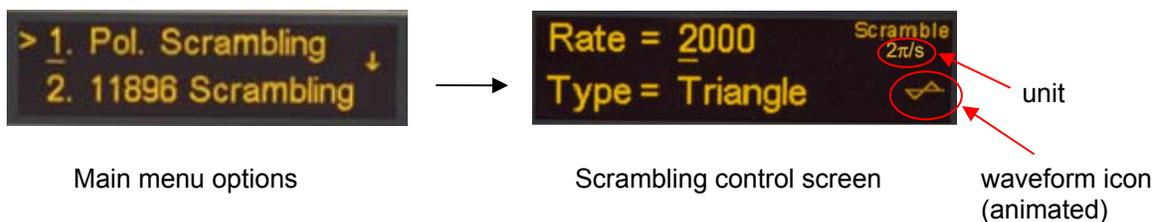
The scrambling control screen has two settable parameters: scrambling rate and scrambling type. To change the scrambling rate, use the ◀▶ buttons to move the cursor and rotate the wheel to change the value of the underlined digit. Press ENTER to switch to type selection. Either use the ◀▶ buttons or rotate the wheel to change the type setting. Both rate and type setting changes are applied in real time as the values are changed.
