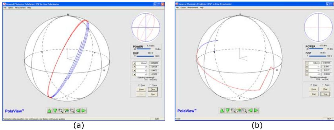
**Figure 21** (a) 150V applied to channel 4. (b) Conversion of a random state to horizontal linear polarization
