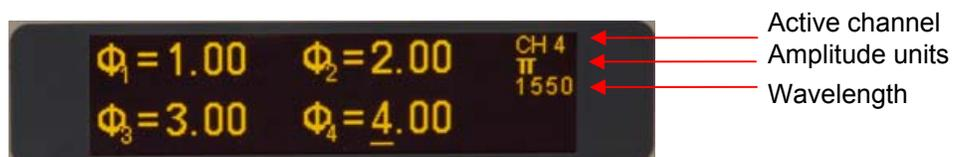
**Figure 19 Manual Polarization Control screen**
