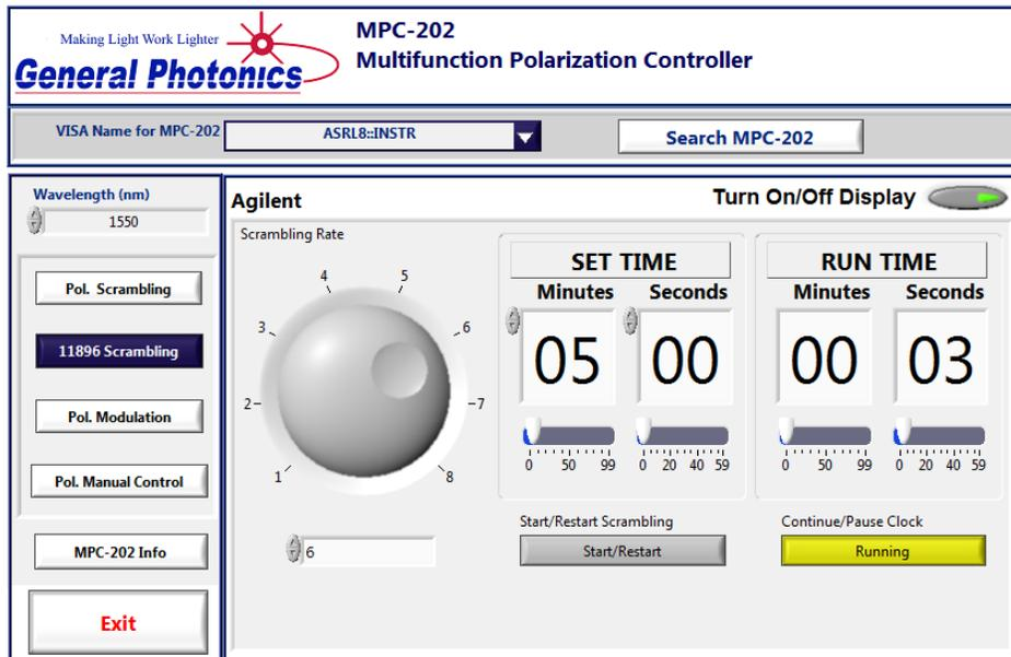
Scrambling rate selection: Adjust the scrambling rate by turning the virtual dial, using the up and down arrows next to the box below the dial, or typing the value into the box and then pressing ENTER on the keyboard.
