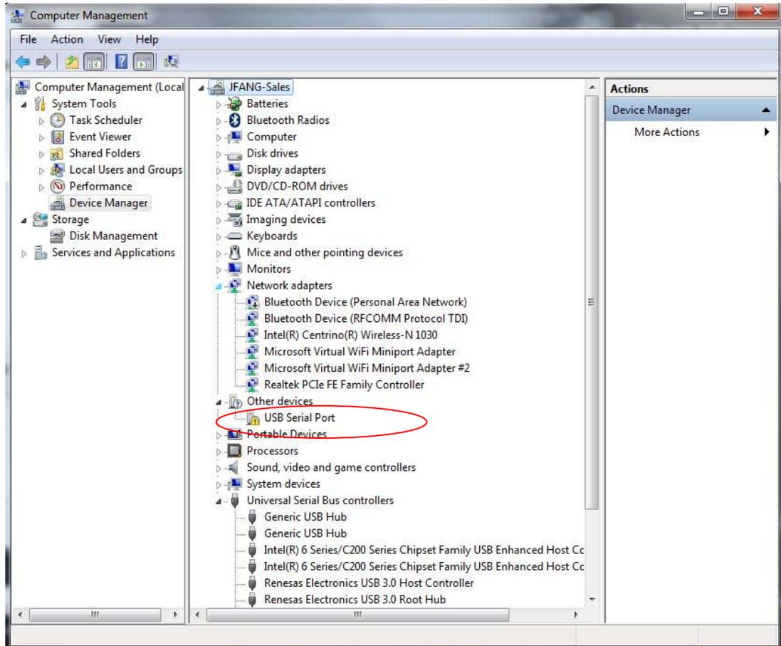
6. In Device Manager, "USB Serial Port" should now appear under "Other Devices". Right-click it and select "Update Driver Software". Follow the same procedure as described above to specify the driver location and install the driver until the completion window for the USB serial port appears:
