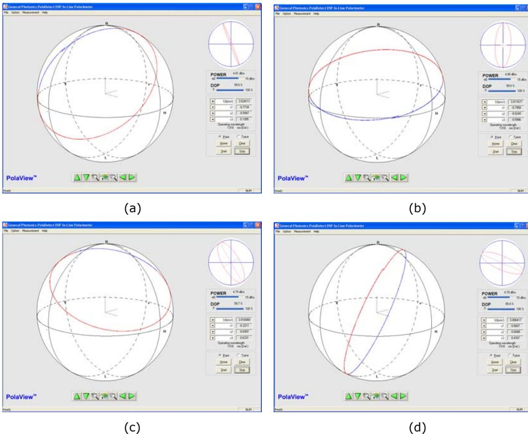
**Figure 20** 0 to 2Vn voltage increase applied to (a) channel 1. (b) channel 2. (c) channel 3. (d) channel 4.
