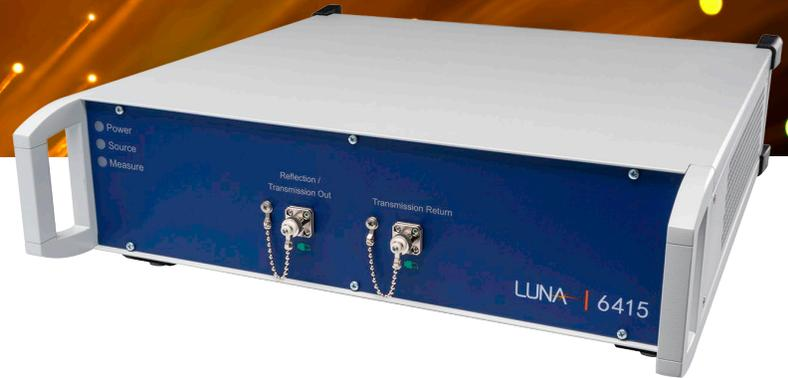
The Luna 6415 Lightwave Component Analyzer is a fast and simple-to-use tool for testing passive optical components and modules. The 6415 measures and analyzes the Insertion Loss (IL) and Return Loss (RL) distribution, as well as length, working in either reflection or transmission mode.
