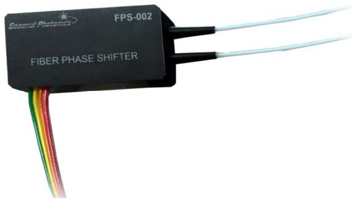
Figure 1 FPS-002 phase shifter
