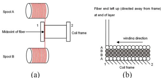
begins from the midpoint of the fiber, and one layer of fiber is wound onto the coil from side 1 to side 2 of the coil frame, using the fiber from spool A. b) Cross section of one quadrupole, which consists of 4 layers of fiber in an ABBA structure.
