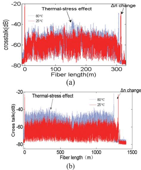
Figure 10 Changes in polarization x-talk of 315 m and 1300 m PMF coils due to thermal-stress effects. (a) 315 m coil (b) 1300 m coil. Solid red lines: measured at 25°C; Dashed blue lines: measured at 80°C. Temperature induced birefringence changes can also be obtained from the location difference of the high x-talk points from the fiber connection points at the far right.
