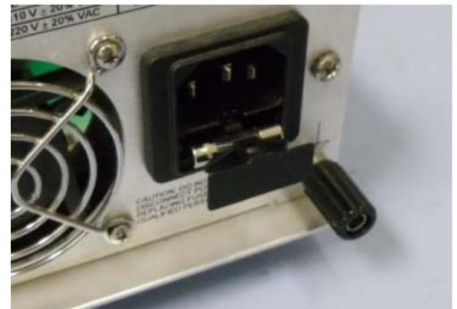
Figure 5 Fuse compartment
