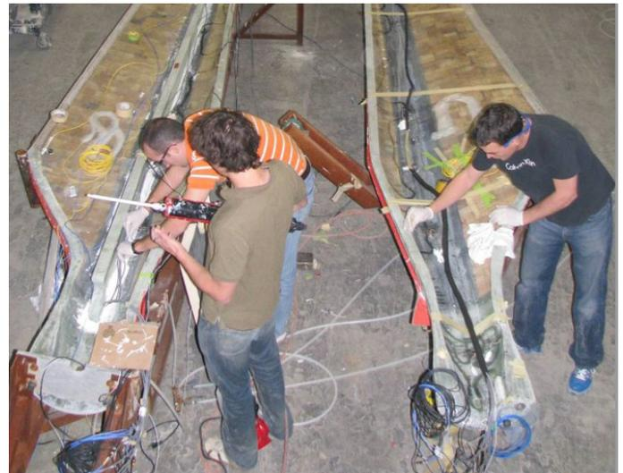
Sensing system installed inside SBlade
