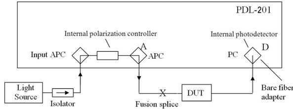
Figure 6 Production floor setup to measure an unconnectorized, pigtailed DUT using fusion splice to a free pigtail and bare fiber adapter to connect to the PDL-201.
