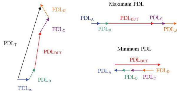
Figure 4 Illustration of the vector summation of PDL contributions from all connectors and DUT. The measured PDL fluctuates between a maximum value and a minimum value, depending on the relative orientations of each PDL vector.
