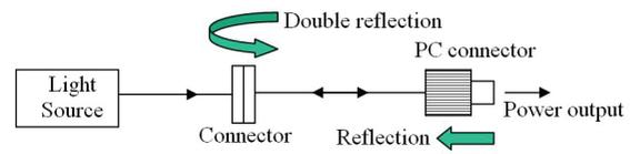
Figure 2 Illustration of double reflection
