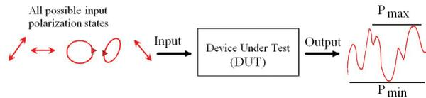
Figure 1 Illustration of PDL definition
