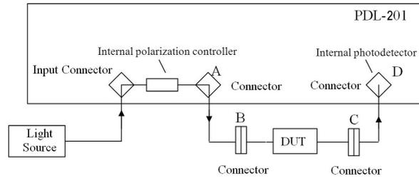
Figure 3 PDL measurement setup using the PDL-201 with 4 connectors: A, B, C, and D
