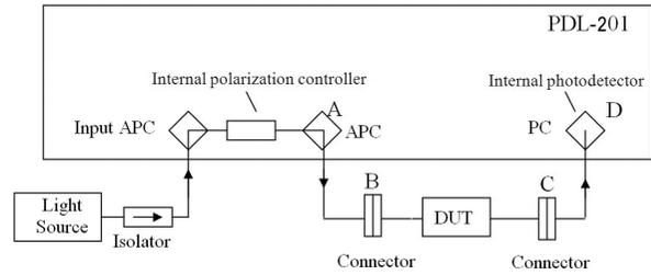
Figure 5 Typical setup for measurement of a connectorized DUT with the PDL-201.
