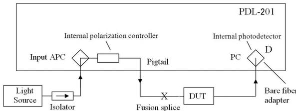
Figure 7 Production floor setup to measure an unconnectorized, pigtailed DUT using only fusion splice and bare fiber adapter to connect to the PDL-201.
