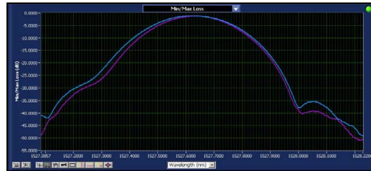
Figure 9-12. The Min/Max Loss plot, showing maximum (blue) and minimum (purple) transmission states.
