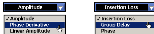
Figure 7-6. The Title Bars , or parameter selection pull-down menus, before and during selection. The left, Time Domain menu is available in the upper and lower graphs. The right, Frequency Domain menu is only available in the lower graph.
