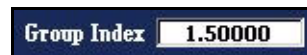
Figure 7-14. The group Index field, which appears when the upper X-axis is set to length.
