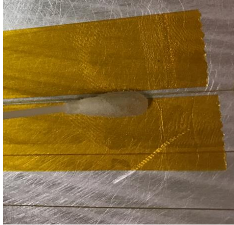
Figure 7: Dispensing epoxy into tape channel on either side of fiber sensor.
